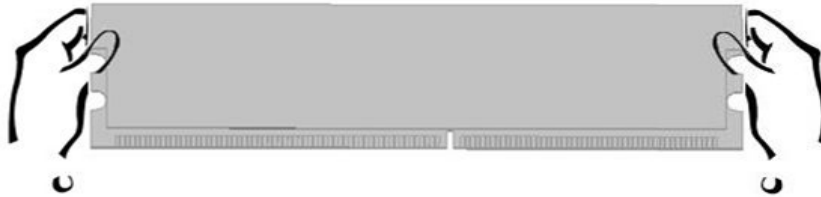
Figure 1 — Example of how to hold module at edges
